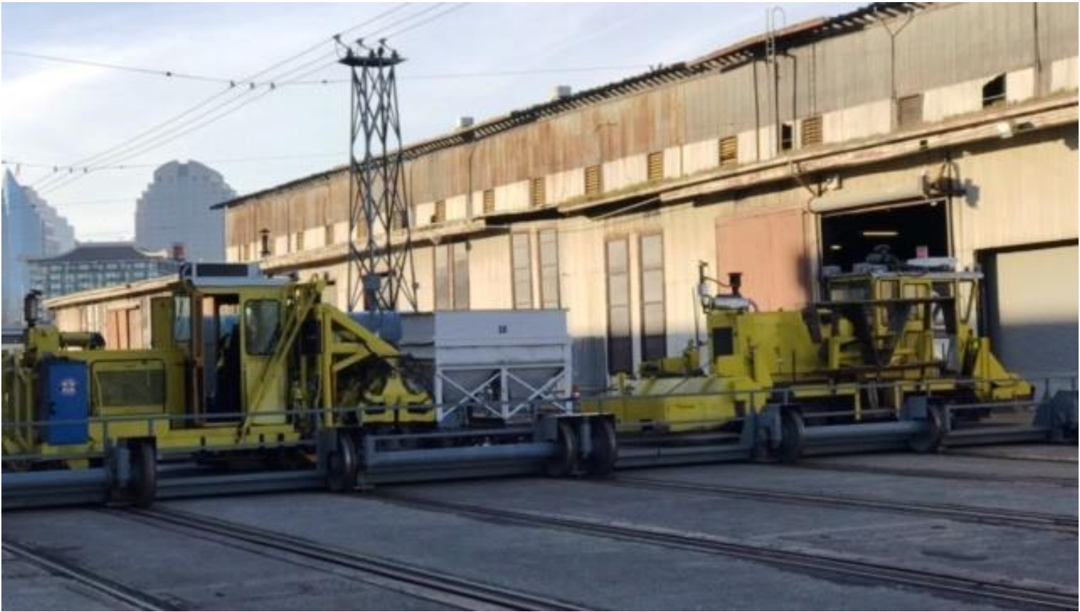
The tamper and ballast regulator are ready to roll – or so we thought...
